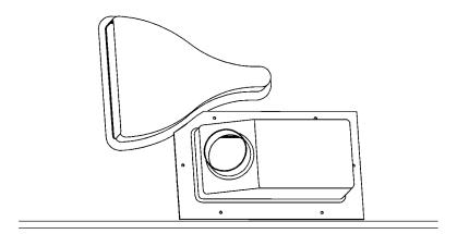
Locate the ACIS air filter housing and retainer on the inside of the bottom tub, passenger side, between the rear air scoop and the strip of reinforcement material which runs fore/aft. Trim as necessary for best fit. When located, drill six 1/8" holes, using clecos to hold alignment. Cut a rectangular opening for air intake (the same size as the inside of the retainer) in the tub.
