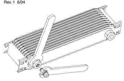
Hose fittings supplied with the oil cooler may vary. If the openings of the cooler have female threads, male adapters must be installed. The fittings that are permanently attached to the cooler must be held with a wrench when installing the adapters and hoses to prevent damage to the cooler.
